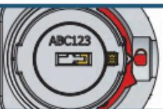
Turn the knob counterclockwise to the „locked“ position.
